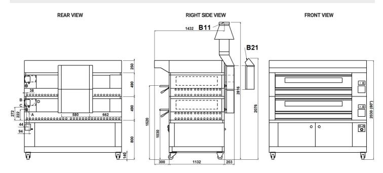
NOTE: The dimensions indicated in the views are in millimeters. B11 DIRECT VENTILATION (ø int 207mm). B21 UNDER VENTILATION HOOD
