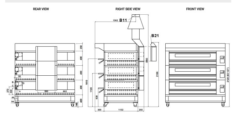
NOTE: The dimensions indicated in the views are in millimeters. B11 DIRECT VENTILATION (ø int 254mm). B21 UNDER VENTILATION HOOD
