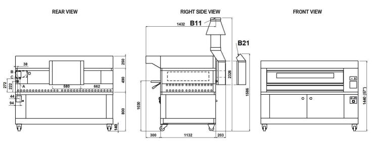
NOTE: The dimensions indicated in the views are in millimeters. B11 DIRECT VENTILATION (ø int 207mm). B21 UNDER VENTILATION HOOD
